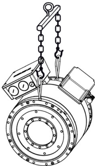
Image 5-1 Lifting and transporting the motor with a cross beam
